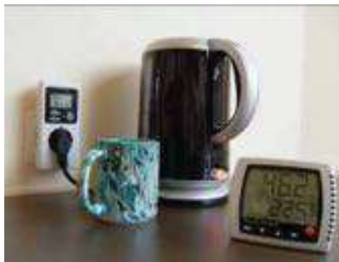
Figure 5. Thermo-hygrometer measures the amount of moisture in the air and the indoor temperature
