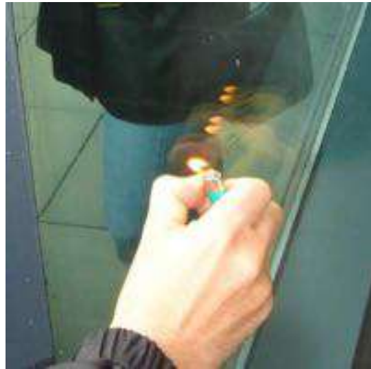
Figure 5. The picture shows the reflection of the light, which is darker and more reddish: this means that the window is coated.
