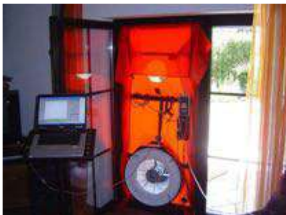
Figure 6. Blower door test (Source: Wikipedia Commons)
