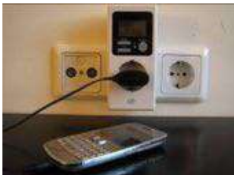
Figure 3. Measuring electricity consumption of electric appliances
